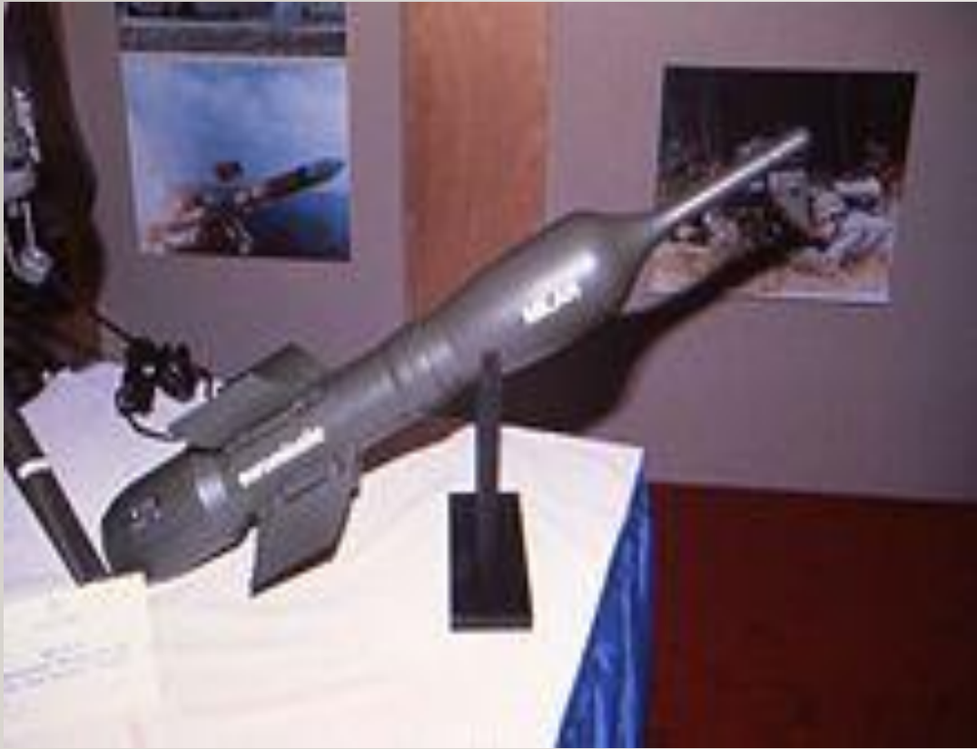
MILAN II with stand-off probe which almost doubled penetration
